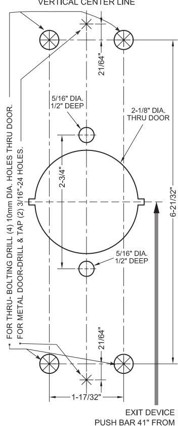
FOR WOOD DOOR-DRILL (4) 3/32" DIA. X 1-1/4" DEEP (WOOD SCREW PILOT HOLES). FOR SEX. BOLTING DRILL (2) 25/64" DIA. HOLES THRU DOOR FOR METAL DOOR-DRILL & TAP (4) 3/16"-24 HOLES. 1/4" 1-1/4" DIA. HOLE WHEN RIM CYLINDER IS USED (LESS OUTSIDE TRIM) **EXIT DEVICE**
