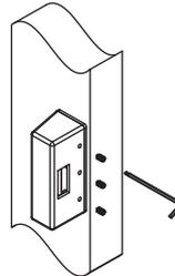
3. Tighten the strike with the M5x10mm set screws using the Allen Key.
