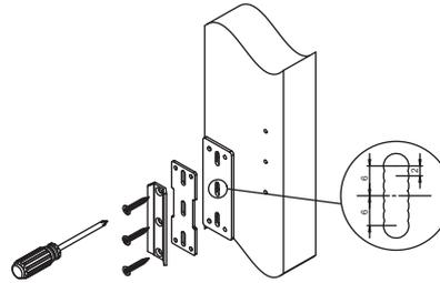
1. Fasten the 3mm Mounting Spacer, Connecting Plate, and Mounting Plate to the door frame using the M5 x 30mm wood screws.
